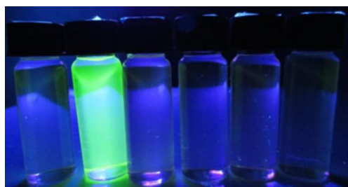
Fig. 6 Six solutions of 11 observed under black light, showing the intense solvatochromism. From left to right: EtOH, HEXN, DCM, MeCN, DMSO, and MeOH
